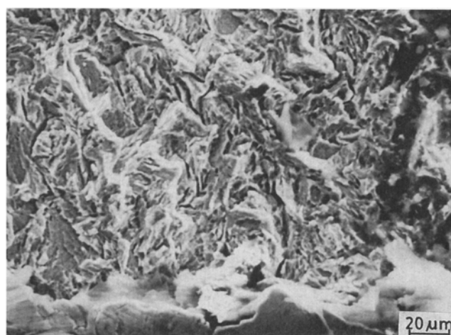
Fig. 5 SEM micrographs of stress-corrosion cracking tested 9Cr-1Mo steel in the normalized condition. (a) Crack initiation by intergranular mode. (b) Final failure by transgranular mode in 0.05 M NaCl medium.
