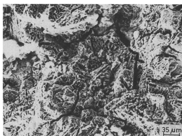
Fig. 6 SEM micrographs of stress-corrosion cracking tested 9Cr-1Mo steel in the normalized condition. (a) Mixed (intergranular + transgranular) mode. (b) Transgranular mode with secondary cracking in 5 M NaCl medium.
